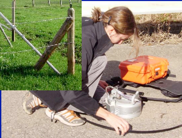
Flux accumulation chamber
